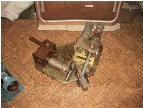
Figure 2 View of the brass-coating device MBZ 3A [7]
